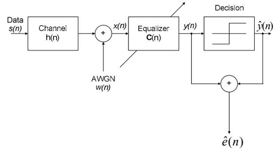
Figure 1. Baseband model of an adaptive blind channel equalization system
